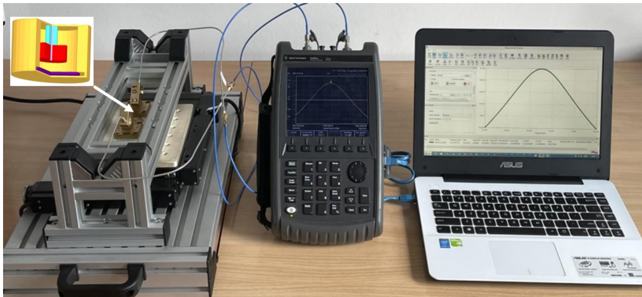
Fig. 3: Photo of an operating setup including 10GHz iSiPDR 2D scanner (left; position of the actual iSiPDR indicated) and Keysight FieldFox (centre) driven by a laptop (right) with QWED control application.
